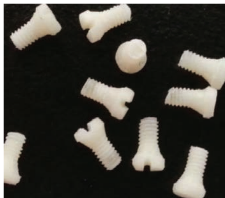
▲ FIGURE 1: Screws made from biologic silk protein.
