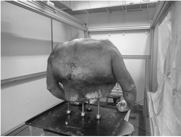
Fig. 1 Specimen A mounted on rod fixture, attached to fixed frame of robotic system, and held in place with volume-expanding foam
