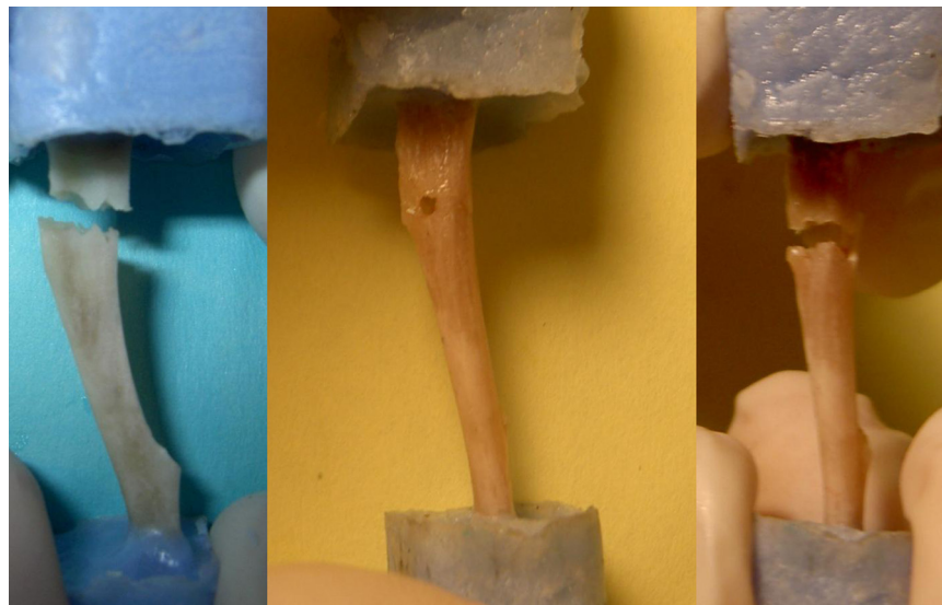
Fig. 3. Three representative images showing fractured tibiae following mechanical testing.
