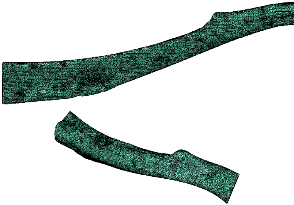
Fig. 6. Finite Element Mesh as presented in a specimen.
