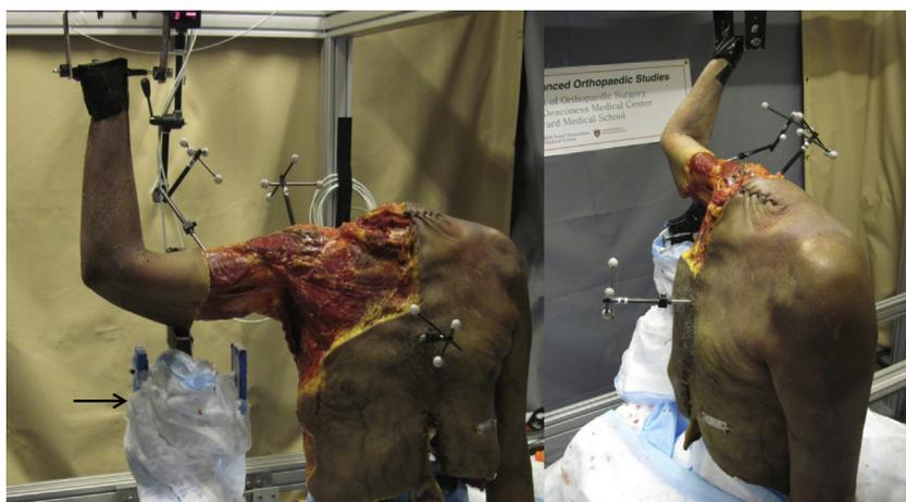
**Figure 3** Torso mounted in test apparatus. The torso is connected to the hand actuator at the level of the wrist to simulate an abbreviated throwing motion. A posterior restraint (arrow) enables full external rotation at the beginning of the motion. Bone markers are used to track shoulder kinematics.
