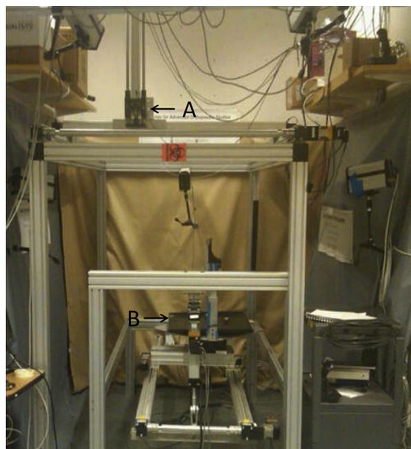
**Figure 1** Testing setup with a lower (smaller) frame and an upper (larger) frame. The actuator (A) of the upper frame can move along the x-, y-, and z-axes, whereas the lower frame (B) can move along the x-, y-, and z-axes and rotate around the y-axis.
