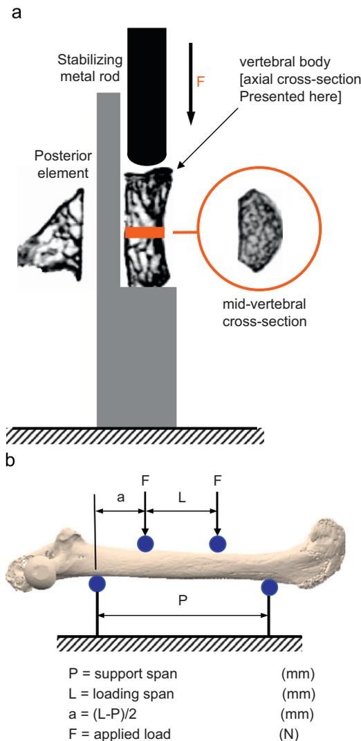
**Fig. 2.** (a) A schematic overview of murine vertebral compression testing. The mid vertebral cross-section is highlighted in the diagram and (b) a schematic overview of murine femoral 4-point bending testing.
