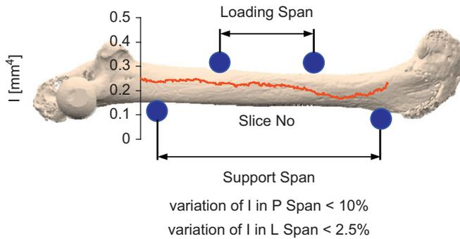
**Fig. 1.** Variation of moment of inertia across the length of a mouse femur, including support and loading spans, with anterior aspect facing down in 4-point bending position.
