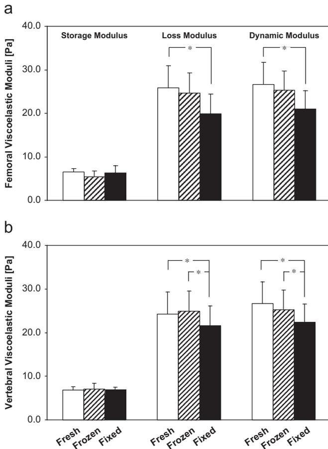
**Fig. 3.** (a) Storage, loss and dynamic moduli for fresh, frozen and formalin-fixed femurs and (b) storage, loss and dynamic moduli for fresh, frozen and formalin-fixed vertebrae. \* denotes  $p$ -values  $< 0.05$ .
