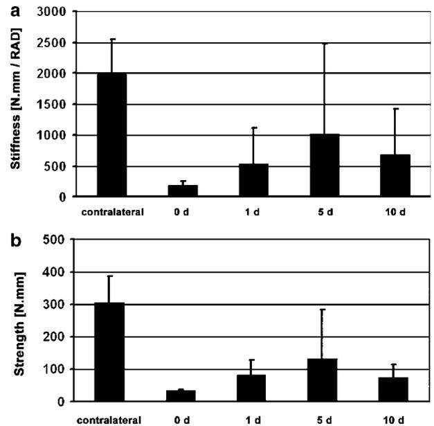
**Figure 7** (a) Stiffness of Ad.BMP-2-treated femora 8 weeks after surgery in comparison to the contralateral, intact femora. Values given are means  $\pm$  s.d. (b) Strength of Ad.BMP-2-treated femora 8 weeks after surgery in comparison to the contralateral, intact femora. Values given are means  $\pm$  s.d.
