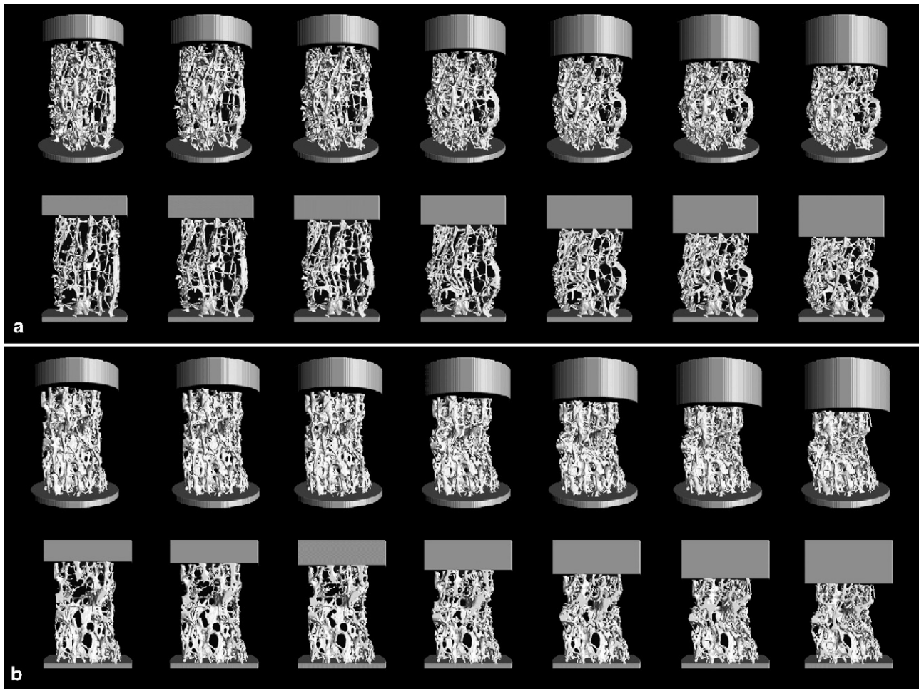
Fig. 1. Compression steps of 0, 2, 4, 8, 12, 16 and 20% global strain from two representative trabecular bone specimens (a and b). The top row, for each specimen, shows a front view of the entire specimen, and the second row demonstrates a representative coronal view of the same specimen viewed from the front.
