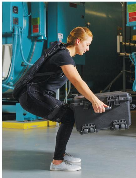
The soft back exosuit by the Harvard Biodesign Lab is designed to relieve some of the strain of heavy lifting.
